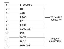
**Figure 6.** MPTAZ115DT, MPTAZ220DT Wiring Diagram for Pan/Tilts and Lenses
